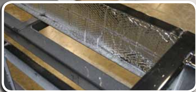
Photo showing 10" I-beam frame rails, fully covered by radiant barrier insulation. NuWa's frames are manufactured locally and are famous for their strength and powder coat finish.
